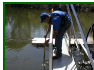
Technician measuring water velocity in front of the mouth of the cone.
