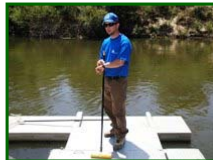
Technician timing revolutions of the cone (i.e. how long it takes for cone to complete 3 revolutions).
